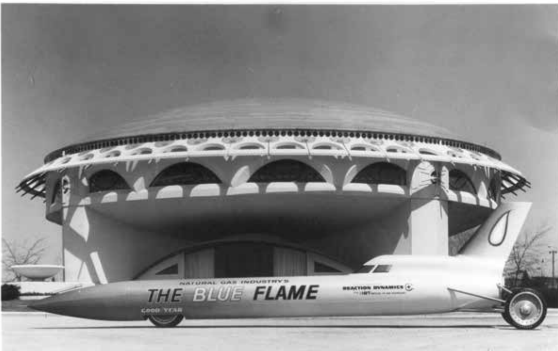
The Blue Flame, shown in front of Frank Lloyd Wright's Annunciation Greek Orthodox Church, was built in Milwaukee by Reaction Dynamics, Inc. Driver Gary Gabelich set the world land speed record in this vehicle at the Bonneville Salt Flats on October 23, 1970, with a speed of 622.407 miles per hour.
